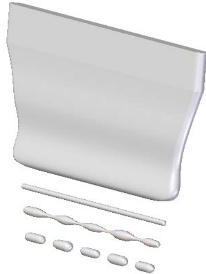
Figure 5: Sketch of a liquid sheet breaking up in transverse strips. This process has not been observed experimentally
